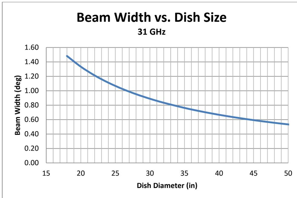
**Figure 2. Half Power Beam width vs. Dish size, 31 Ghz.**
