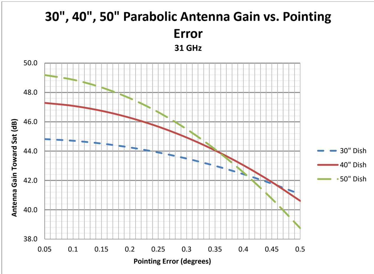
**Figure 4. Antenna Gain in the direction of the Satellite vs. pointing error for 30”,40”,50” diameter dishes, 31 GHz.**
