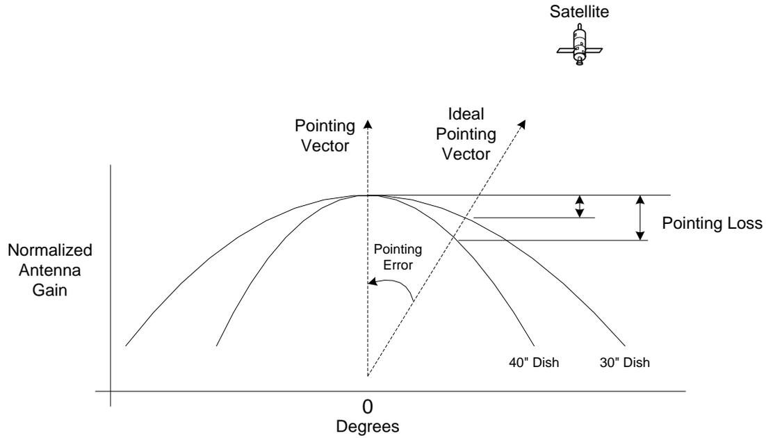
**Figure 1. Normalized antenna gain for two dish sizes, pointing loss increases with larger dish due to narrower beam**
