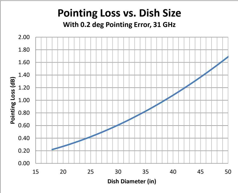
**Figure 3. Pointing loss vs. Dish size for a 0.2 degree pointing error, 31 GHz**
